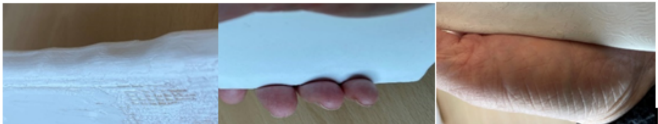
Figure 4: An impression of the 3d printed rounded form at the edges (left), the position of the fingers for the right handed phone in the indents (middle) and the position of the thenar in the double handed phone (right).
