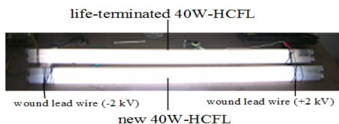
Figure 31: Photopictures of lighted 4 coil-EEFL lamps in parallel connection under the DC external driving circuit. Two FL lamps (above) are converted from life-terminated 40W-HCFL lamps taken from scrap yard. Two FL lamps (below) are converted from new 40W-HCFL lamps from store.
